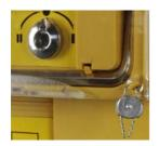
The transparent cover can only be sealed when it is closed (automatic mode).
