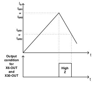
Fig. 1: Meaning of switching recovery level
