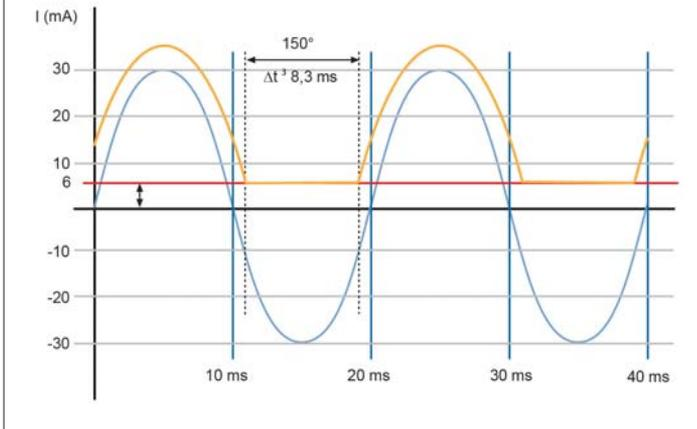
As a result of the joint discussions, the topic of monitoring DC fault currents  $I_{\Delta n} \geq DC 6 \text{ mA}$  arose. Residual current devices of type A in accordance with IEC 61008-1/IEC 61009-1 are only designed to trigger in case of sinusoidal or pulsating fault currents. In case of direct fault currents in the range  $I_{\Delta n} \geq DC 6 \text{ mA}$ , both the response time and the response value can be degraded on the usage of type A residual current devices (Figure 5).
